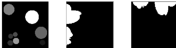
Fig. 3. A discrete image and its horizontal and vertical projections (from left to right, respectively).
