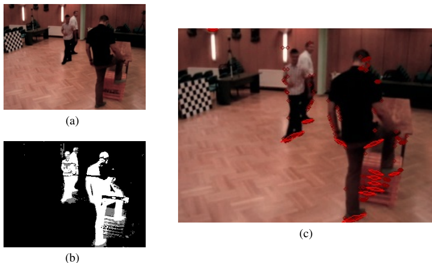
Fig. 1. Shadows may corrupt foreground detection even in carefully chosen color space. Foreground mask (b) for an input frame (a) is shown, as well as the resulting feet points and ellipses (c) (ellipses are visualized with lozenges). A number of false positives are introduced due to corrupted foreground mask.
